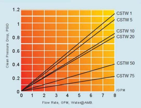
Flow rate is per 10" cartridge. For liquids other than water, multiply the pressure drop by the fluid viscosity in centipoise
