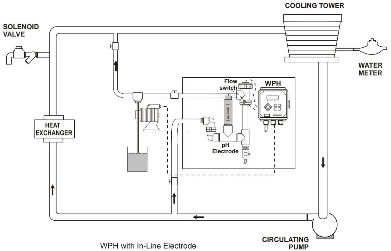
Figure 1 Typical Installation
