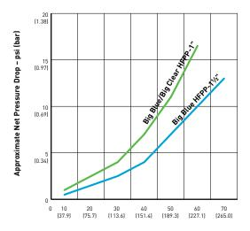
Flow Rate - gpm (Lpm)
