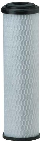
**The Pentair<sup>®</sup> Pentek<sup>®</sup> C8 Series Cartridge offers an economical solution for general purpose water filtration needs. Constructed of a carbon impregnated cellulose media, this dual-purpose cartridge filters chlorine taste & odor, bad taste & odor and sediment particles\*. The cartridge has a high dirt-holding capacity and can be used in a wide variety of applications.**
