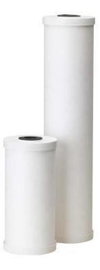
Pentair<sup>‡</sup> Pentek<sup>‡</sup> RFC Series Cartridges are constructed with a 70-micron porous polyethylene outer shell and durable polypropylene endcaps. The 2-3/4" outer diameter cartridges have a polypropylene core and the 4-1/2" outer diameter cartridges incorporate a spun polypropylene core. Sandwiched between the outer shell and the core is a bed of granular activated carbon (GAC).
