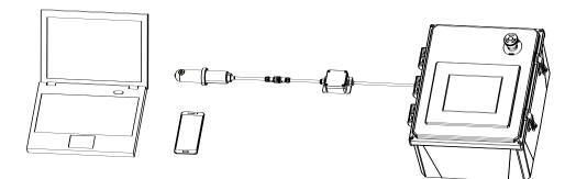
Figure 1. ST-500 connected to computer or smart phone via WiFi/Bluetooth/Wif adapter
