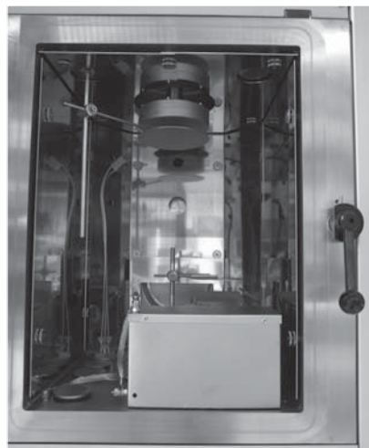
Rotating and water-cooled substrate table
