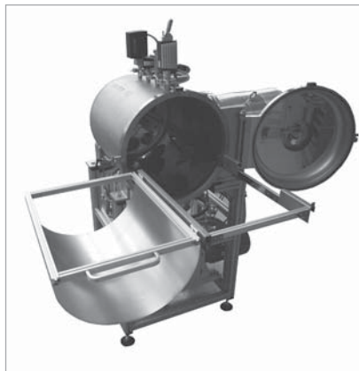
Opened coating chamber with retracted substrate receiver
