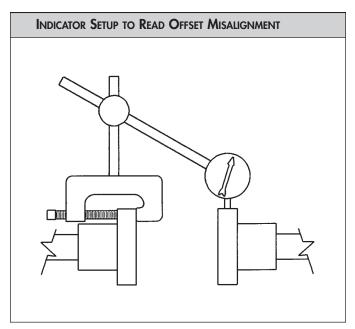
To check the offset alignment, mount the dial indicator as above except with the indicator button on an outside diameter of the stationary coupling hub. Rotate the shaft on which the dial indicator is mounted, allowing the indicator button to ride on the outside diameter of the stationary hub. The indicator dial movement will show the difference in the center locations of the two shafts. Good practice suggests alignment to within 0.002" T.I.R.
