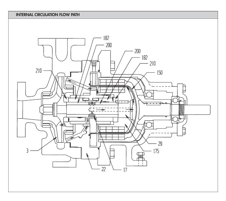
The internal circulation flow path through the bearings and the magnetic coupling is supplied with discharge pressure and returns to discharge pressure. The differential pressure required to do this is supplied by an impeller built into the outer end of the inner magnet assembly (175). This flow provides cooling to the magnets (175) and the containment shell (150) and also lubrication as well as cooling to the bearings (182), journal sleeves (200) and thrust collars (210).
