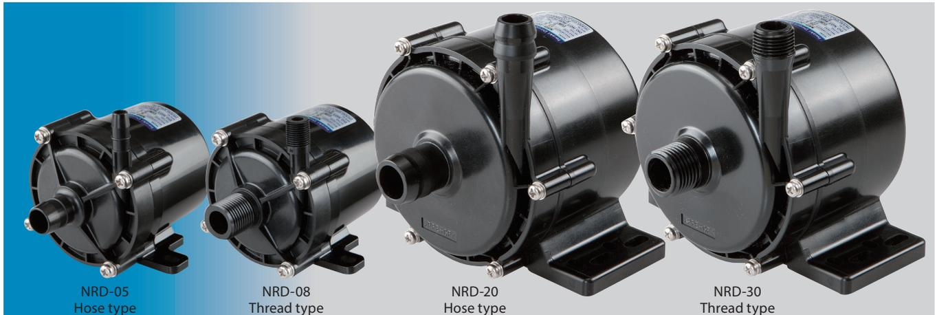
Our NRD series design features small canned motor centrifugal pumps powered by brushless DC motors. They are incredibly compact, lightweight and quiet. A variety of features, including a seal-less design to prevent leakage, enable the pumps to meet a full spectrum of user needs, with emphasis on ease of installation, operation and maintenance.
